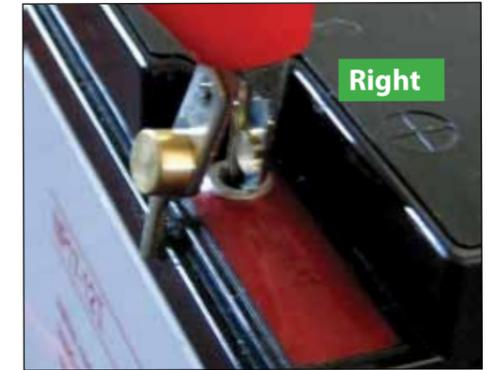
Push clips tightly inside battery terminals
